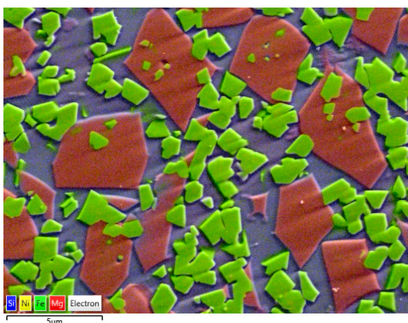
Fine scale microstructure with faceted iron oxide and olivine grains in a silicate-rich matrix collected from the Winchcombe meteorite using Ultim Max 170 for 90 seconds at 5 kV. Sample courtesy of UKFALL
